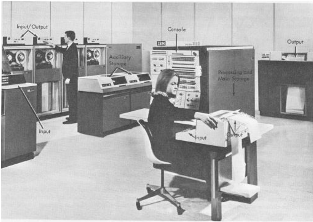
Figure 9 Shows an IBM System 360 Model 40 data processing System
