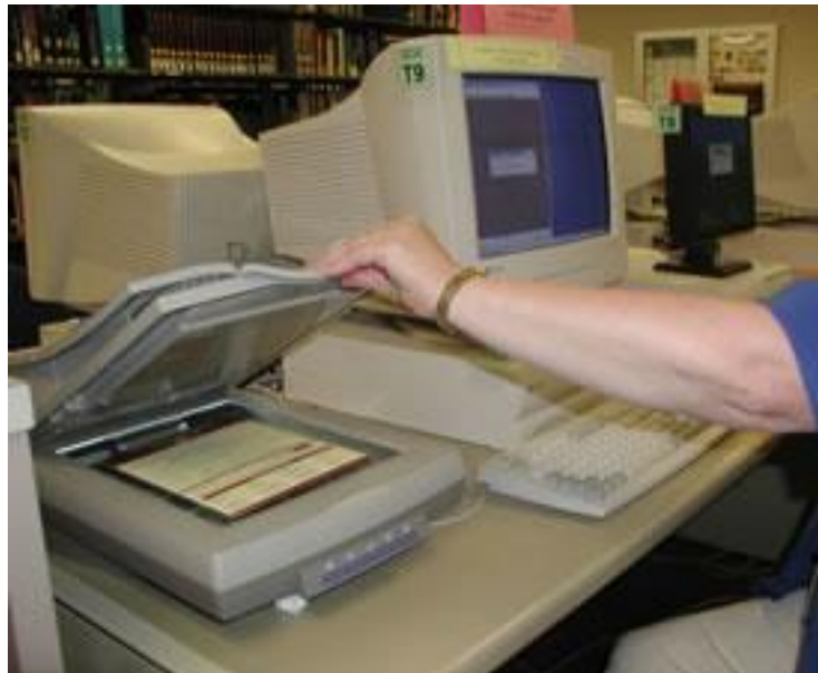
Figure 1 Shows a Scanner. This device is connected to the computer. Any photos you have in your hand can be converted into electronic form using this device. Software would be needed to process the data from the Scanner.
